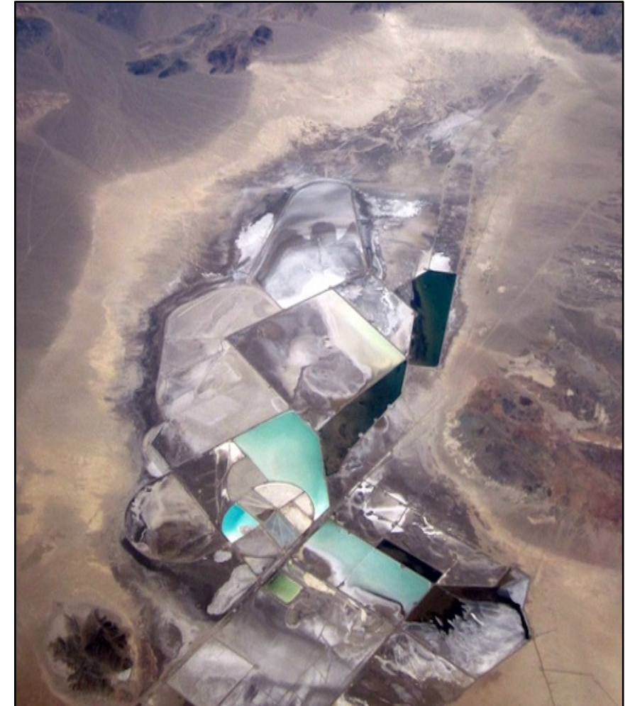
Lithium-brine evaporating ponds at Clayton Valley, Nevada
