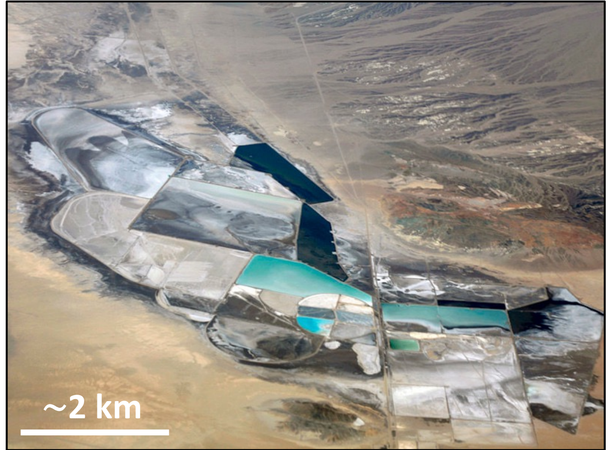
Lithium-brine evaporating ponds at Clayton Valley, Nevada (Albemarle)
